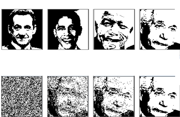
Figure 4: Experiment 1A, connectivity: 32 random connections. The upper row shows the individual stable states as they appeared in the 98x98 weightless neuron network. The lower row shows the time development (left to right, t=0, t=1, t=2, t=4) of the system starting in a random state and ending in one of the four experienced states.
